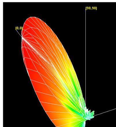
Figure 10: 3D Radiation pattern of 8-element linear array
